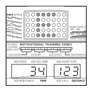
the + button. While an E or an M appears in the matrix, the left display will show the total numbers of hours that the elliptical crosstrainer has been used, and the right display will show the total number of miles pedaled. When you are finished viewing this information, press the Start Program button again.
